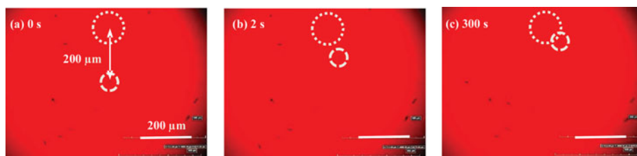
Figure 4. Photo-induced manipulation of glass rods on a PEG film doped DR1 ( 7.5 \times 10^{-5} mmol/mg in PEG). The time-bar marked on the pictures is the irradiation time. The circle in fine imaginary line is the irradiation area; the circle in bold imaginary line is the position of glass rods.
